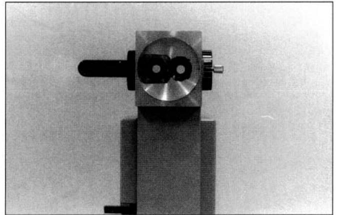
**Figure 2:** The pocket for the barrier filter (A of Fig. 1) as seen from the observation system by detaching the latter. The light entering through an objective lens is split into two equal beams. The pocket for the barrier filter was added to the left side leading to the angiographic camera.
