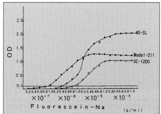
Figure 5: Effective density range in response to fluorescein (optical density OD).
