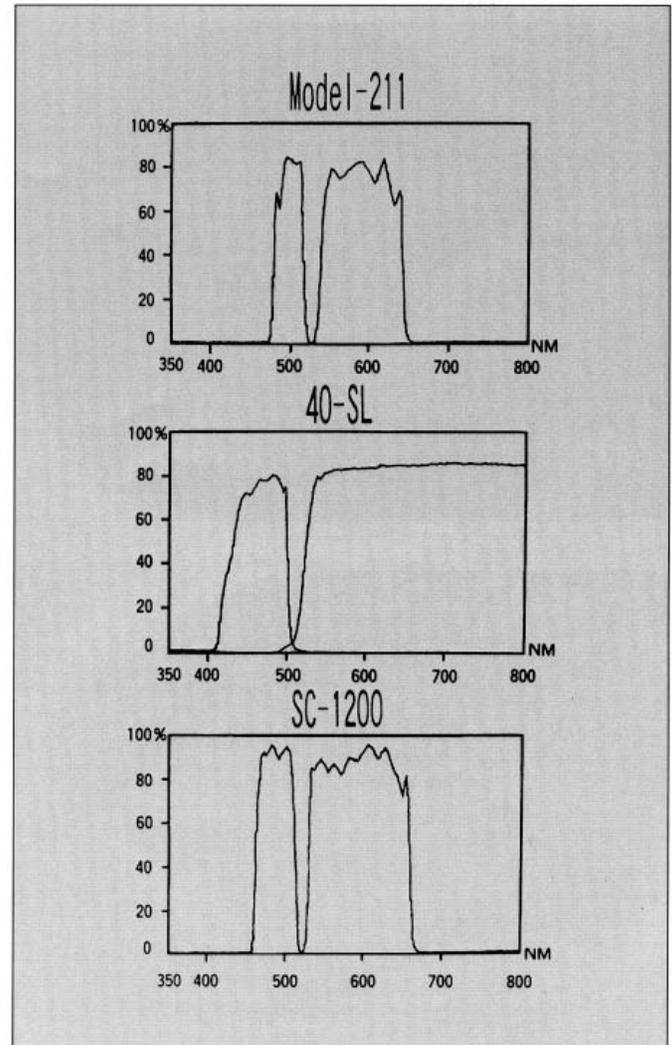
Figure 4: Comparison of the filter characteristics of each device.
